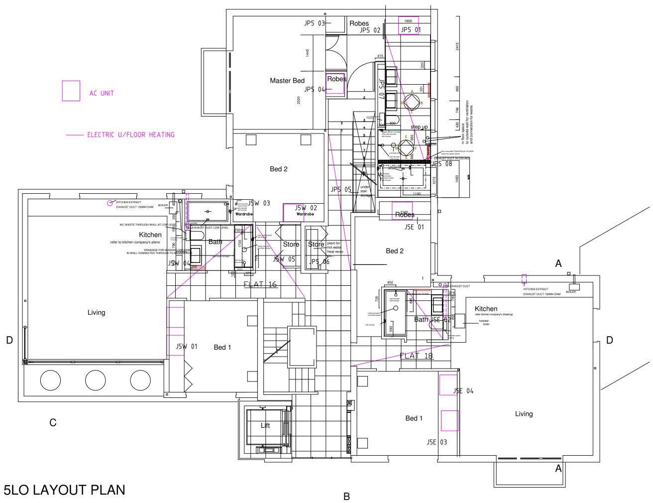
FIFTH FLOOR AC FANCOIL POSITIONS & ELECTRIC U/FLOOR HEATING BATHROOMS & EXHAUST DUCTS
